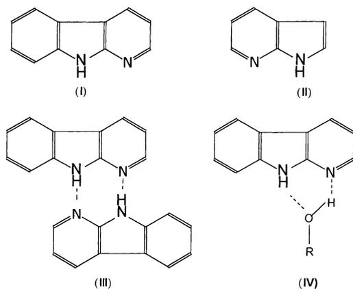
Fig. 1. Structural formulae of AC (I), 1-AI (II), the AC dimer (III) and the doubly hydrogen-bonded cyclic complexes of AC.
